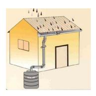
and storage of rainwater into natural reservoirs or tank. One method of rainwater harvesting is rooftop
